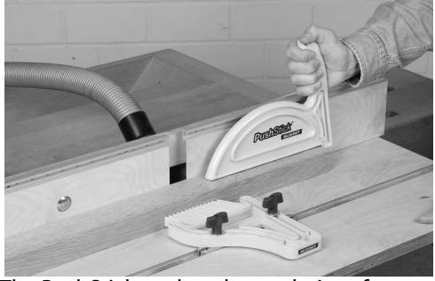
The PushStick pushes the workpiece forward while providing downward pressure against the table.
